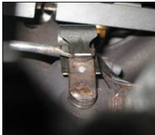
Figure 3. Wastegate linkage with clip in final position.
