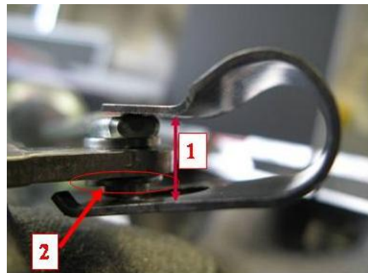
Figure 8. (2) Position of the original circlip.
